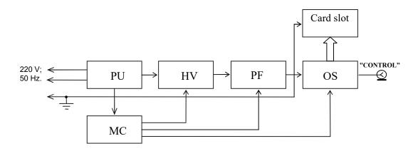
Fig. 1 The functional chart of the test generator IGE Sc
